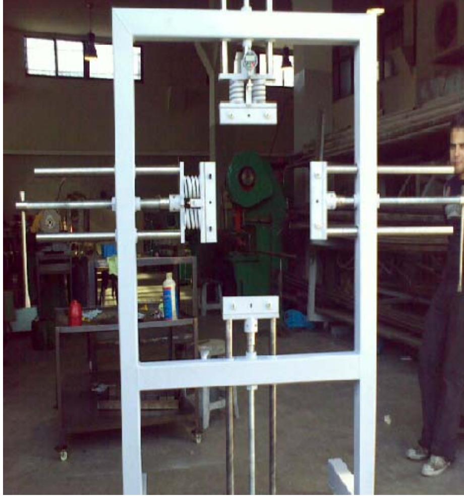
Figure 4.7: photo of manufactured biaxial loading machine for carrying out the experimental verification.
