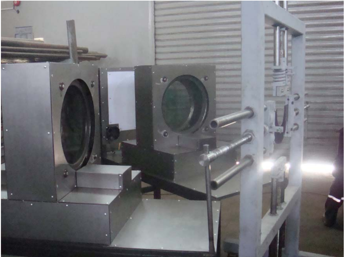
Figure 4.6: photo of reflection polariscope setup that is manufactured for experimental verification.
